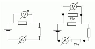
Placing voltmeter and ammeter in a circuit and the effect of their internal resistance
