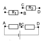
Two resistors or other devices, elements of the circuit are connected *in series* when they are joined at one end but no other element is connected to their joining point. The free ends of the joined elements are connected into the circuit.
